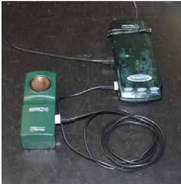
To begin with, make sure your motion sensor and LabPro sensor hub are connected. They should already be plugged in for power and connected to the computer via USB. If not, plug the motion sensor into one of the digital ports on the left side of the LabPro hub. The LabPro should be connected to one of the available USB ports on the computer and plugged into the power outlet on the bench.
